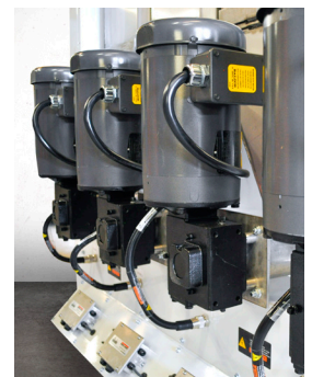
Close up of the motor gearbox, & junction box
