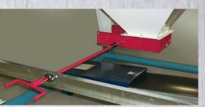
The rack & pinion gate has an extended control rod for easy operation.
