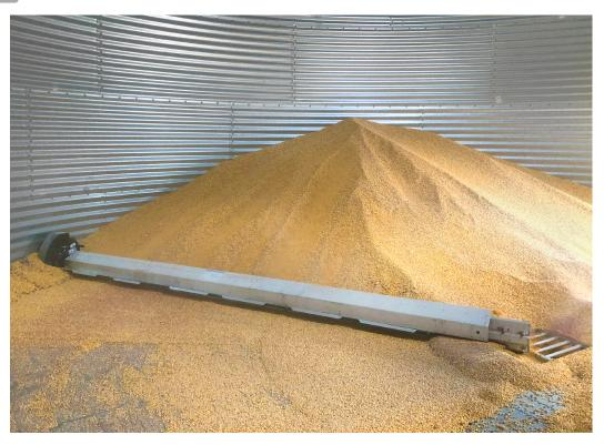
**Sweep carrier:** Standard on all sweeps in bins 54' and larger. Wheel design helps spread the weight on bin floors.
