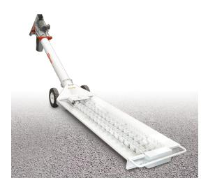
Need to move fertilizer fast? The Railcar Unloading Hopper has tons of experience with just that. The Ox FH-500 and FH-510 Railcar Unloading Hopper can unload granulated fertilizer from hopper bottom cars at speeds up to 40 TPH. Its low-profile leaves plenty of clearance and its well-balanced design makes it easy to maneuver. It's rough, it's rugged, and its special corrosion resistant paint makes this one tough hopper.
